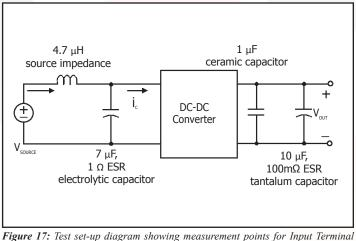
Figure 17: Test set-up diagram showing measurement points for Input Termina Ripple Current (Figure 9) and Output Voltage Ripple (Figure 10).
