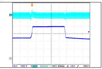
*Figure 12:* Output voltage response to step-change in input voltage (1000 V/ms). Ch 1: Vin (100 V/div), Ch 2: Vout (200 mV/div). Horizontal Scale: 1 ms/div
