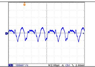
**Figure 10:** Output voltage ripple, Vout, at nominal input voltage and rated load current (100 mV/div). Load capacitance:  $10 \,\mu F$  tantalum capacitor. Bandwidth: 20 MHz. See Figure 17. Horizontal Scale:  $2 \,\mu s/div$
