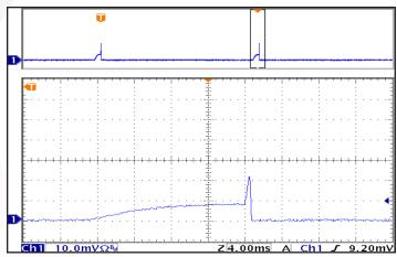
**Figure 18:** Load current (50 A/div) as a function of time (4 ms/div and 100 ms/ div) when the converter attempts to turn on into a 10 m $\Omega$  short circuit.
