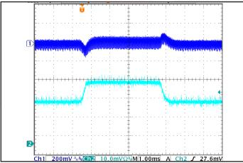
**Figure 11:** Output voltage response to step-change in load current (50%-75%-50% of lout(max); dI/dt = 0.1 A/µs). Load cap: 1 µF ceramic and 15 µF tantalum capacitors. Ch 1: Vout (200 mV/div), Ch 2: lout (20 A/div). Horizontal Scale: 1 ms/div
