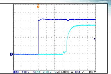
*Figure 8: Turn-on transient at full resistive load and zero output capacitance initiated by Vin. ON/OFF Pin previously low. Ch 1: Vin (100 V/div). Ch2: Vout (2 V/div). Horizontal Scale: 40 ms/div*
