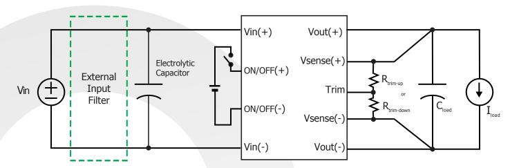
Figure D: Typical application circuit
