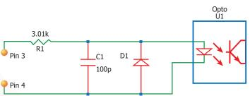
Figure B: Internal ON/OFF pin circuitry
