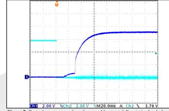
*Figure 7: Typical startup waveform from enable pin at full resistive load. Input voltage pre-applied. Ch1: Vout (2 V/div), Ch2: Enable Pin (2 V/div). Horizontal Scale: 20 ms/div*
