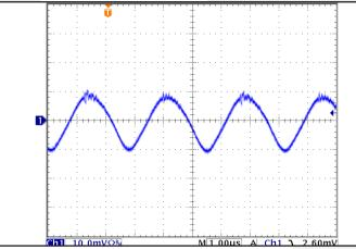
**Figure 9:** Input terminal current ripple, i<sub>c</sub>, at full rated output current and nominal input voltage (200 mA/div). Bandwidth: 20 MHz. See Figure 17. Horizontal Scale: 1 µs/div
